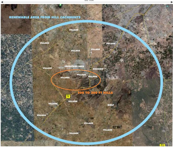
The renewable ground water area from traps in the hills could extend 25 kms in a circle as indicated in blue on the satellite image from 35KM altitude. The hills run in an L shaped path for approximately 7 KM and have an altitude ranging from 200 to 300 feet above the manesar area which lies approximately 750 feet above sea level..
