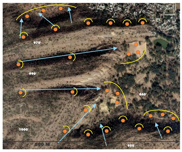
The example area is approximately 800 meters across imaged from an altitude of 3200 feet. The blue arrows indicate possible rain water flow paths, we have a flow descent of approximately 160 feet. We have envisaged a requirement of approximately 30 shallow bore holes and about 500 Meters of check walls
